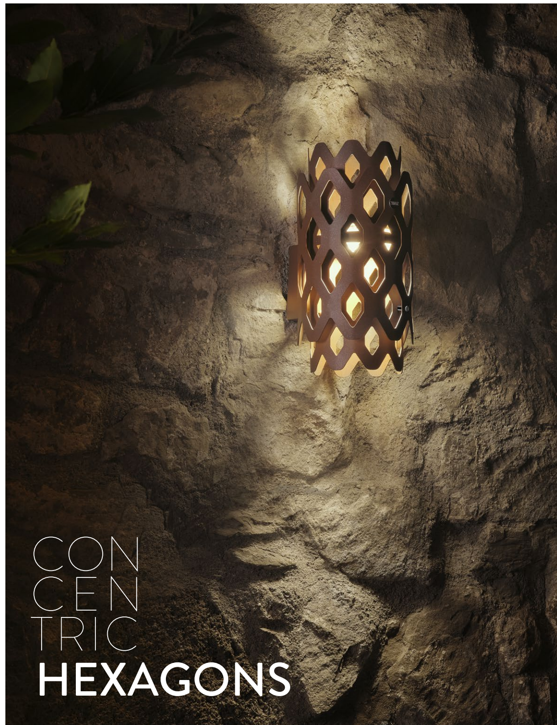
Charlotte Applique technicals: Lighting: 4.2W - 220~230Vac/50Hz - 500 Lumen - 3000 Kelvin - IP65 - Bidirectional LED (110V version available). Dimension: 14 x 17 x h 28 cm
